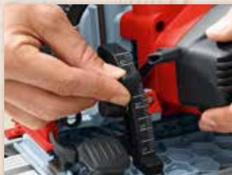
Thanks to the unique tilting system, a cutting depth of 47 mm (including rail) is always available in the angle range from 0° to 45°.
