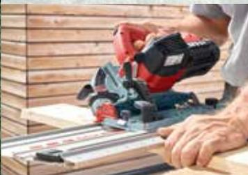
Thanks to the generously-sized angle scale and precise double clamp, miter cuts can be realized that ensure a perfect fit - as illustrated here on exterior cladding.
