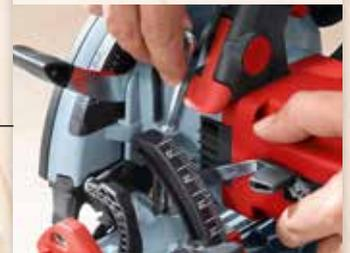
The K 65 cc's cutting depth can be preset and locked in the range from 8 to 67 mm.
