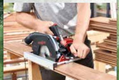
Using the MAFELL guide tracks or the parallel fence included in the delivery scope, which is graduated in millimeters, decking boards for instance can be made to fit exactly.
