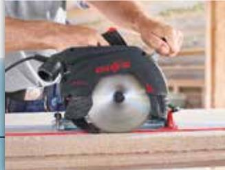
Dispensing with a detachable riving knife, the FLIPPKEIL permits reliable, convenient and straight-forward plunge cutting.
