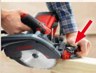
The pivoting guard is retracted quickly and easily by means of a lever for convenience and safety when executing bevel and plunge cuts.
