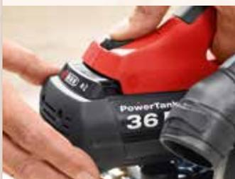
Pressing the battery release button interrupts the power supply and automatically locks the sawblade. The blade can then be changed safely and without risk with the Allen key attached to the machine.
