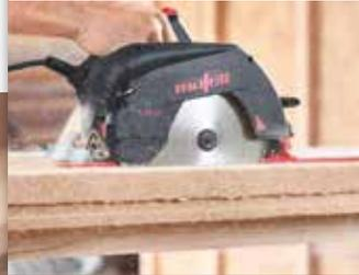
The chip management system was designed and optimized for cutting fiberboard. The superb chip removal system offers substantial benefits, including when executing plunge cuts in the fiber direction.
