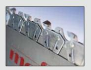
The new ZSX-TWIN Ec carpenter's chain saw is a highly practical tool for large timbers.
