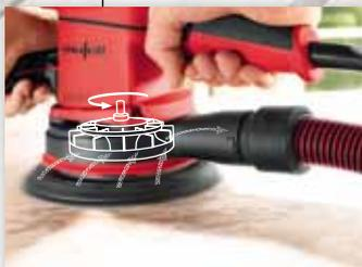
In combination with the multi-perforated sanding pad, powerful self-extraction creates a low-dust and safe working environment. As a consequence, the abrasive disc is less prone to clogging, disc life is prolonged, and work outcomes are improved.
