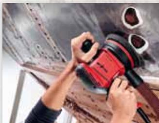
For coarse sanding, the EVA 150 E/5 is the ideal choice. The 5 mm stroke and a speed of 12,000 rpm represent the perfect combination for this kind of work.
